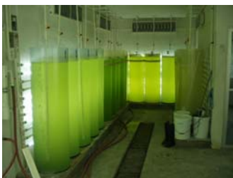
Figure 2: Fiber glass carboys for Dunaliella viridis reproduction.
