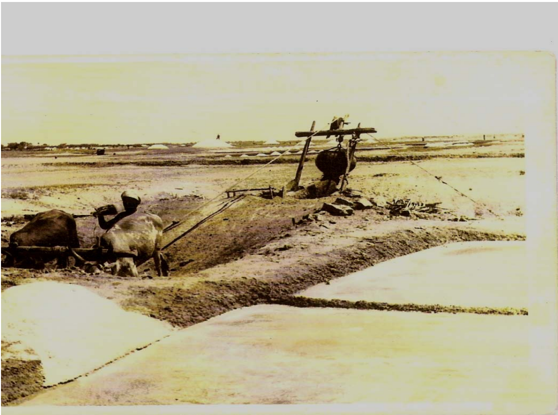
Method of brine lifting - using pair of bullocks.
